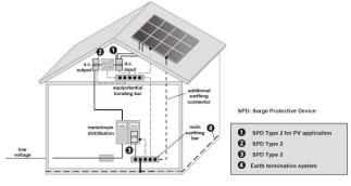
Figure : installation of various SPDs on photovoltaic application
