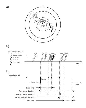
Figure : Example of an alarm. a) Locations of the lightning related events in the defined areas (coverage area CA, monitoring area MA, surrounding area SA, and target ); b) temporal occurrence of the lightning related events and c) timing of the alarm according to the occurrence of the lightning related events
