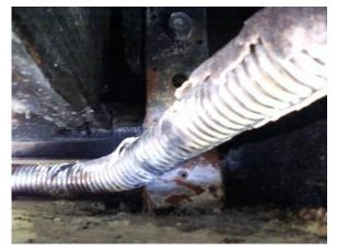
Figure 1. Location of CSST Damage Near a Strap Connected through a Concrete Footing
