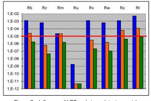
Figure 7 – Influence of LPS and storm detector on risk parameters in example N°1
