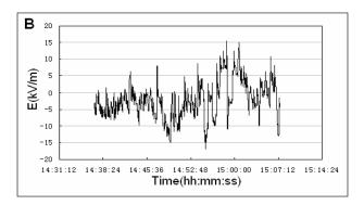
Figure 4 – Variation curve of electric field observed in Jiuting Town during two different periods
