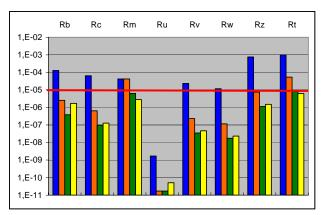
Figure 8 - Influence of LPS and storm detector on risk parameters in example N°2
